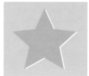
*Effect of misregistration when the bottom object is knocked out*
